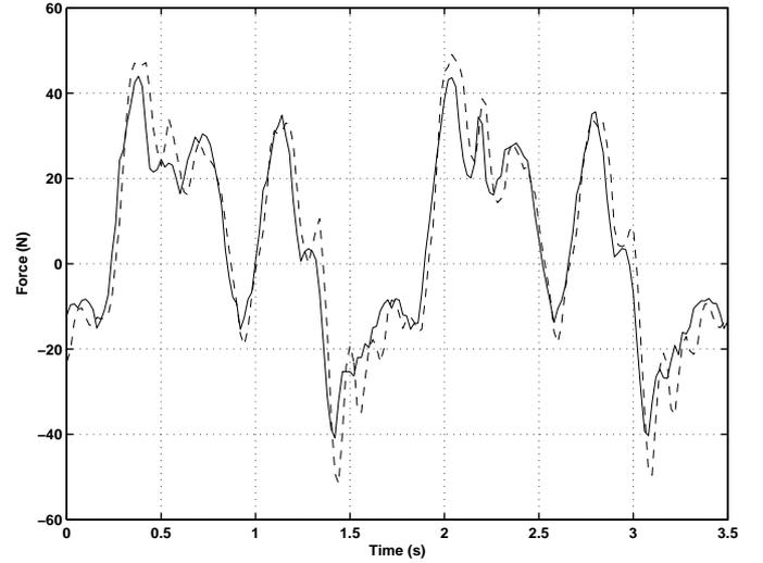
Figure 5. PNEUMATIC ACTUATOR FORCE TRACKING DURING THE TEACH-AND-PLAY. SOLID LINE: DESIRED FORCE, DASHED LINE: ACTUAL FORCE.
