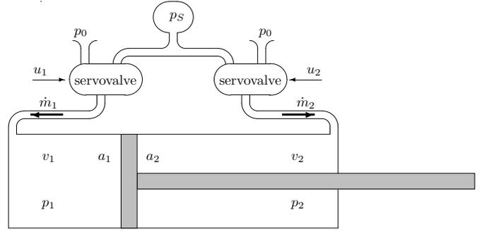
Figure 4. SCHEMATIC DIAGRAM OF A PNEUMATIC CYLINDER.
