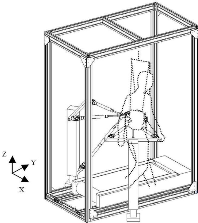
Figure 1. CONCEPTUAL DRAWING OF PELVIC ASSIST MANIPULATOR (PAM).
