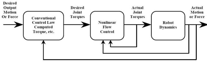
Figure 3. HIERARCHICAL NONLINEAR PNEUMATIC CONTROL LAW.
