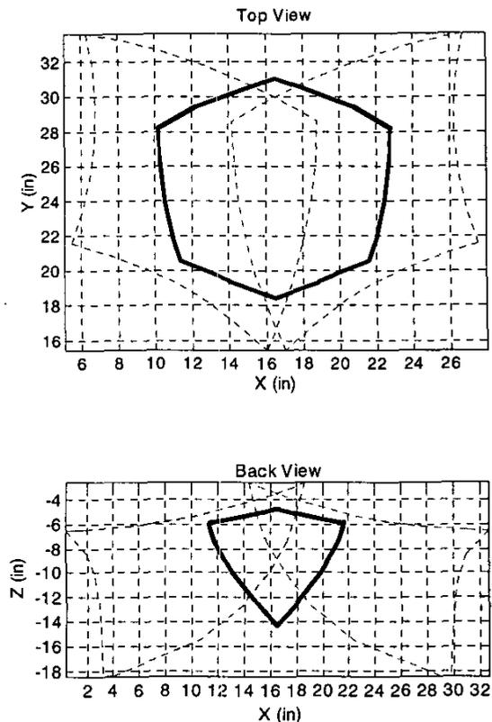
Fig. 3 PAM workspace. Dotted lines: Individual, uncoupled robot workspaces of left and right belt attachment points; Solid line: Workspace of the belt center-point that will allow  $\pm 6^\circ$  of planar angular displacement, i.e. during normal walking speeds, of the belt in the assembled system (max belt angular displacement is about  $\pm 20^\circ$ ). Coordinate frame shown in Fig. 1 originating at the ball-joint of the posterior, horizontal cylinder.
