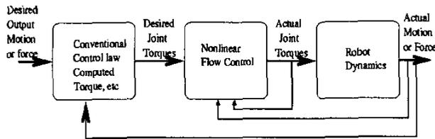
Fig. 2: Hierarchical, Nonlinear, Pneumatic Control Law
