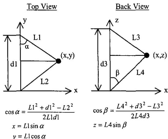
Fig. 4. Forward kinematic equations to infer the position of the cylinders to belt attachment point  $(x, y, z)$ .
