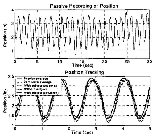
Fig. 5. A: Passive motion capture data of a subject's lateral hip displacement over a 30-second interval on a treadmill moving at 2 mph. B: Position tracking of the calculated average step trajectory from the data in Fig. 5A for three cases, along with that average of the passive motion capture data and also the average of a zero-force control motion capture data over a 5-second interval. Subject was a 23-year-old, 200 lbs., unimpaired male. Supply pressure was 85 psi.
