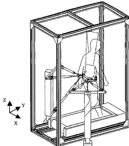
Fig. 1 Pelvic Assist Manipulator (PAM). Two three-degree-of-freedom pneumatic robots are mounted on adjustable pillars and attach to the back of a belt worn by the subject.
