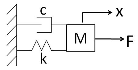
In lecture we modeled the vibrating beam as the system shown above. That is, we modeled as a mass-spring-damper system with a force input F.
