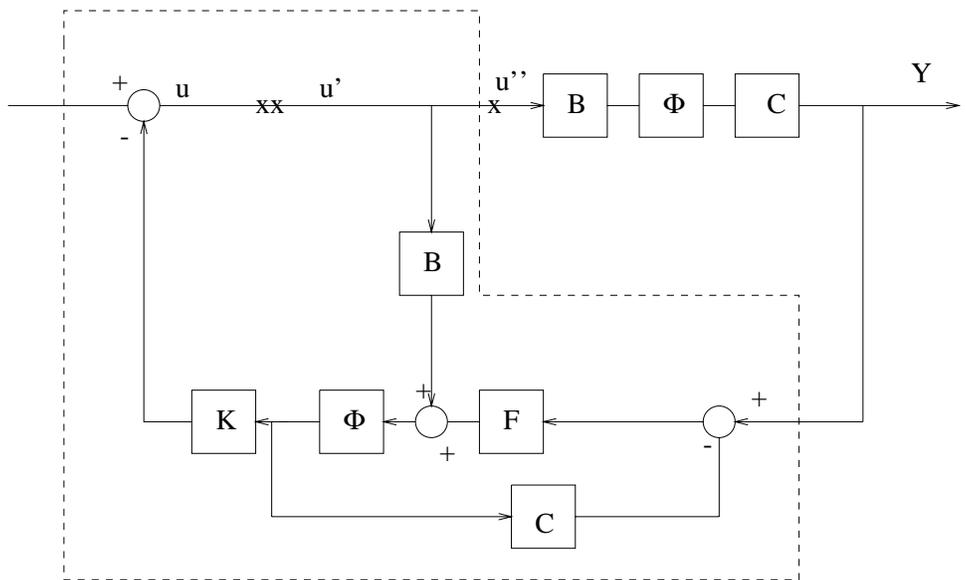
Figure 9.2: Block diagram for the observer based controller
