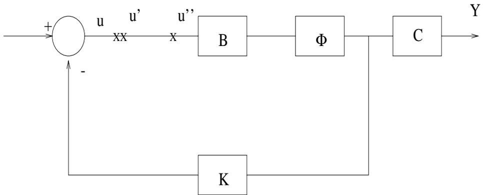
Figure 9.1: Block diagram for the full state controller
